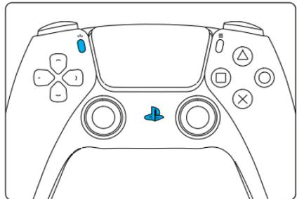
Example: Initial pairing for PS5 DualSense - Press Share + PS button for several seconds until the touch bar LEDs flash rapidly
